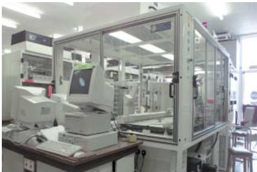
Figure 3. A view of part of the autopurification system: the linear track ORCA® robot plate-handler (Beckman Coulter, Fullerton, CA, USA) is housed in a recirculating safety cabinet. The MS and evaporative light scattering unit are situated below the bench on the right-hand side. Some of the eight semi-prep HPLCs can be seen in the background.
